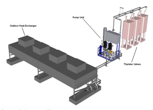
Example: Cooling system, Water to Air
