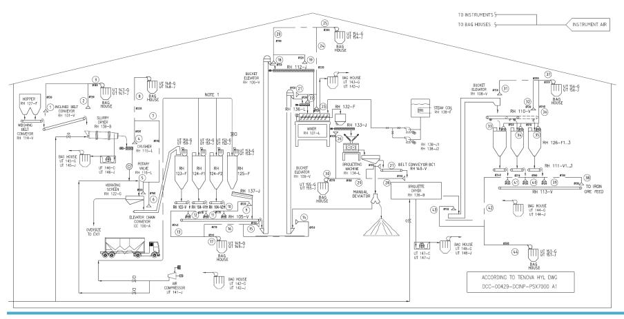
Figure 10.4-28.: Flow diagram of the briquetting plant
