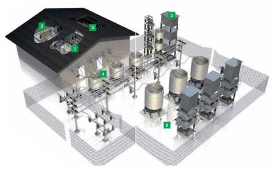
1. VSC | 2. Control and protection system | 3. Cooling system | 4. Phase reactors |
