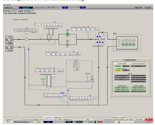
Example: Cooling system visualization in HMI
