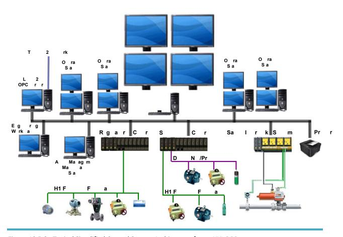
Figure 10.5-2.: Typical Simplified Control System Architecture for an HYL DRP
